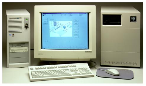
The Arachne portable web inspection system consists of a Windows NT system running Arachne Analysis Software, a VME-based real-time disk, and the Black Widow inspection engine (pictured above).
