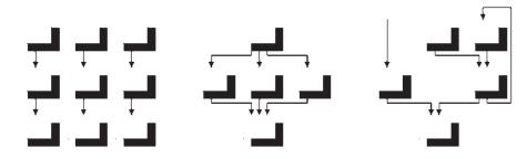
Like an assembly line, data in a pipeline processing system passes through a series of specialized computational elements that are connected sequentially. In addition, these elements can be reconfigured on the fly to accommodate countless numbers of application-specific processing needs.
