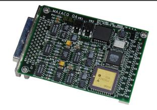
Video inputs for up to four cameras/sensors per converter (eight inputs total)
