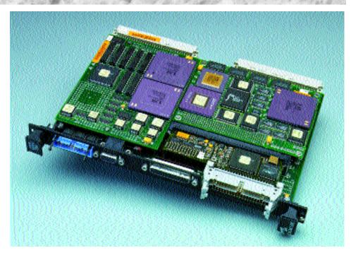
The MaxVideo 250's built-in Analog Gener-ator provides a programmable display and graphics overlay for a variety of resolutions and outputs including gray-scale, pseudocolor, and true color.
