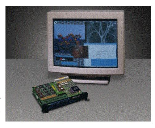
The 24+8 True Color model, 24-bit plus 8-bit overlay (1280x1024 @ 76 Hz), is used for true color display or double- or triple-buffered grey-scale image display. The top of the line 24+8 Turbo True Color model, 24-bit plus 8-bit overlay (1600x1280 @ 76 Hz), also offers two simultaneous 120 MB/second inputs from the image processor.
