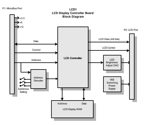
LCD1 controllers accept pixel coordinates in direct H and V values. ALU hardware enables them to perform pixel set, clear, and XOR operations, or byte write and byte XOR operations. The result is that drawing operations are fast and efficient. Figure 1 is a block diagram for LCD1. The table below shows which panels are supported by each version
